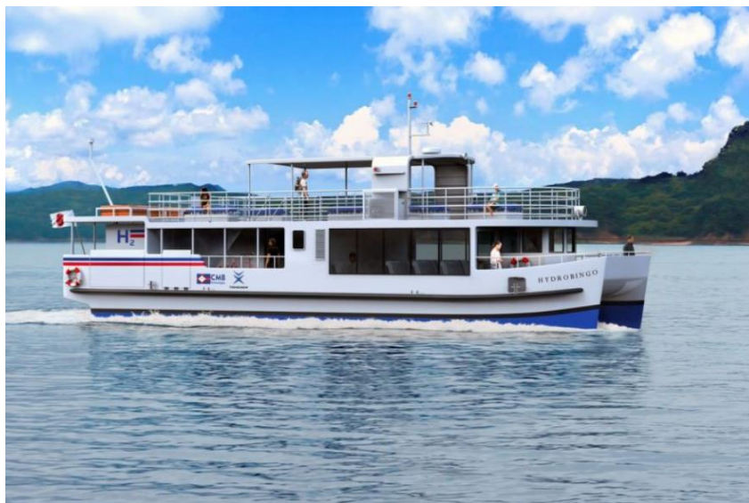
Figure 6.7: Hydrobingo - the first hybrid diesel/hydrogen ferry for commercial use
